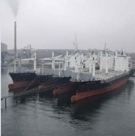
Typically vessels are either laid up in "hot" or "cold" mode. Hot lay-ups are short term allowing the vessel to return to service at short notice. Cold lay ups are for a longer term that requires the vessel to be moored in a secured location and all systems are shut down. In either case, it can be expected that the fuel will degrade during the lay-up period, with sediments settling and asphaltenes flocculating resulting in excessive sludge build-up in fuel tanks and handling systems.
